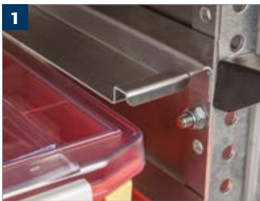
1 Rails with stops keep CarryLites in place during transportation.
